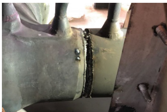
Fig. 4. Arc gouging results for defective weld. Source: Images made by the authors
