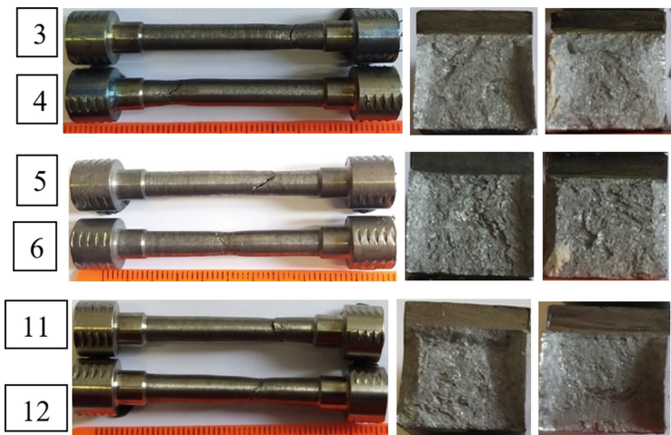
Fig. 3. Most typical failure types for permanent connection coupons from VT20 titanium alloy versus EBW conditions and post-weld heat treatment with numbers specified in Table 2. Source: prepared and compiled by the authors
