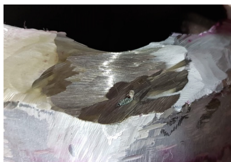
Fig. 13. Slag inclusion in base metal. Source: Images made by the authors
